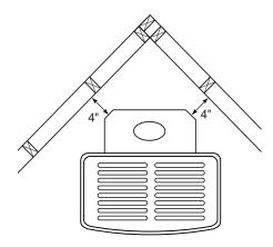
Figure 4 - Clearance for Corner Installation
